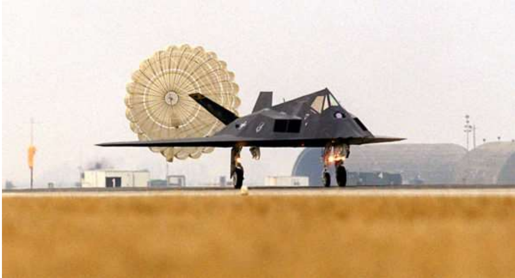
Figure 10 : Lockheed F-117A stealth attack aircraft having deployed its braking parachute at a US base in Italy [US department of defence 1999 ]
