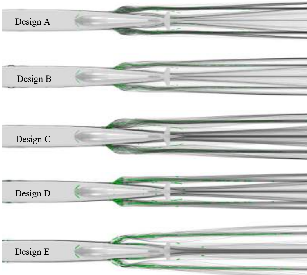
Figure 45 : Streamlines and vortices downstream of the vehicle for a 223.52 \text{ m}\cdot\text{s}^{-1} speed
