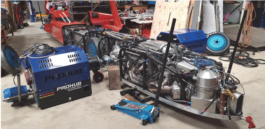
**Fig. 3 The Wairua 2 streamliner vehicle shown during construction and dyno testing (December 2023).**
